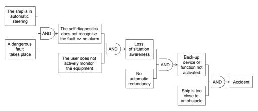
Figure 1. The event-tree presentation of a typical accident after a failure in a safety-critical automation system
